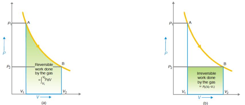
(a) The reversible work of expansion; (b) The irreversible work done by the gas when the external pressure is at once dropped to the final value  $P_2$ .
