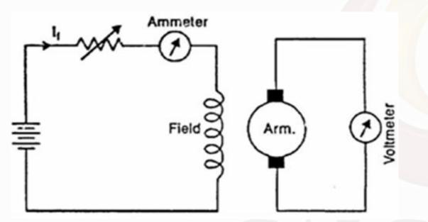
OA – Due to residual magnetism AB – R<sub>i</sub> is negligible and R<sub>g</sub> is constant BC – B is high. Hence R<sub>i</sub> increases
