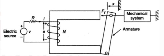
• Mechanical energy output = Electrical energy input – Stored field energy  $F_f dx = i d\lambda - dW_f - - - - 8$
