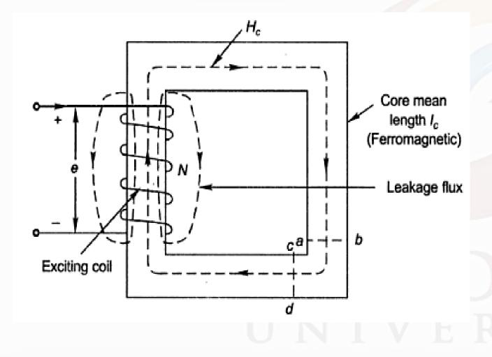
Electromagnetic system Ferromagnetic core **Exciting coil** Coil has N turns Coil carries a current of I amps Magnetic field established Magnetic flux flows through the core Small flux leaks through air
