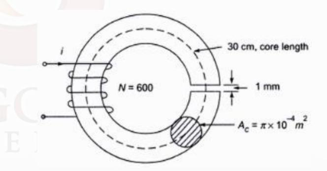
(i) No Air-Gap  $N.i = H_c l_c$  $i = \frac{0.5 \times 10^{-3} \times 30 \times 10^{-2}}{600.\pi (1 \times 10^{-2})^2 (4\pi \times 10^{-7}) \times 4000}$  $N.\,i=\frac{B}{\mu_0\mu_r}\,l_c$ i = 0.158 A $N.\,i=\frac{\phi.\,l_c}{A.\,\mu_0.\,\mu_r}$  $i = \frac{\phi \, l_c}{N \, A \, \mu_0 \, \mu_r}$
