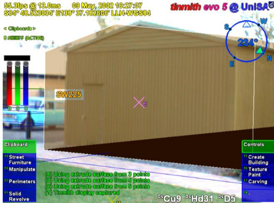
Figure 8 - AR view showing building model with sloped roof registered against the physical object
