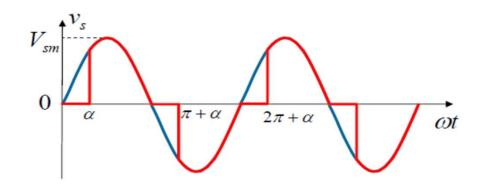
$$V_{0rms} = \sqrt{\frac{1}{\pi} \int_0^{\pi} v_L^2 d\theta} = \sqrt{\frac{V_{sm}^2}{\pi} \int_{\alpha}^{\pi} \sin^2 \theta \cdot d\theta}$$
