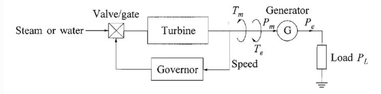
When there is a load change, it is reflected instantaneously as a change in the electrical torque output *Te* of the generator.
