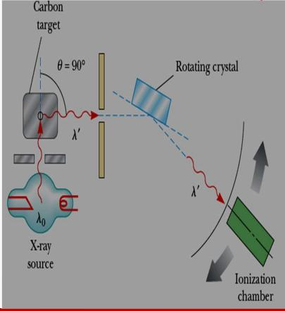
Here X- ray photons are scattered through 90° from a carbon (graphite) target. The wavelength is measured with a rotating crystal spectrometer using Bragg's Intensity of the law. scattered X-rays are the measured using ionization chamber.
