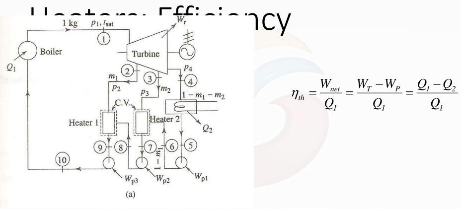
$$W_T = 1(h_1 - h_2) + (1 - m_1)(h_2 - h_3) + (1 - m_1 - m_2)(h_3 - h_4)$$
