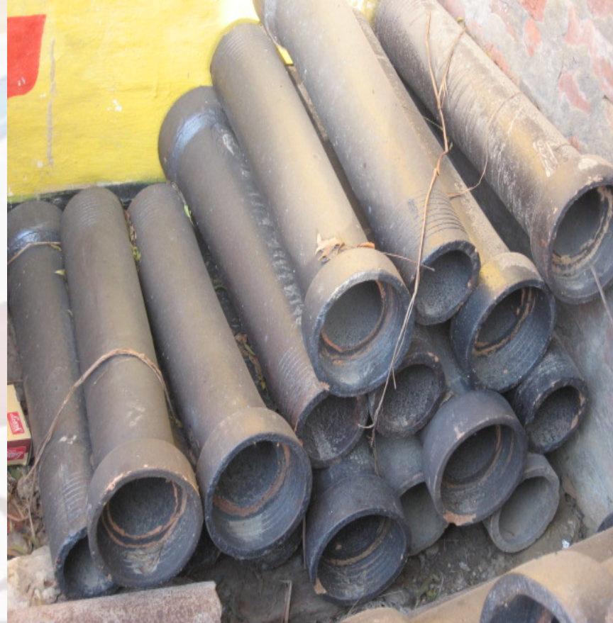
6 inch dia SW PIPES
