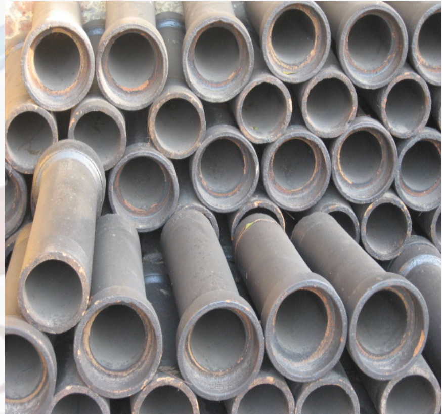
4 inch dia SW pipes
