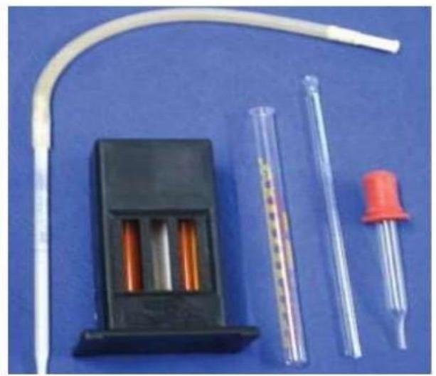
L-R: Pipette Sahli's Standard Hemometer Tube Stirring Rod Dropper
