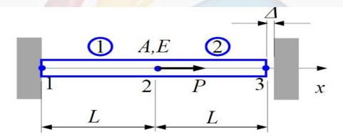
*Problem*: Determine the support reaction forces at the two ends of the bar shown above, given the following,
