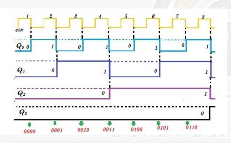
4-bit Ripple Counter Using JK Flip flop – Time Diagram
