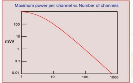
• In a long haul system with periodic amplification, SNR performance in presence of Raman scattering has been estimated. If the acceptable decrease in SNR in the channel with smallest wavelength is 0.5dB, the number of transmittable channels N can be calculated using  $n(n-1) = \frac{8.7 \times 10^{15}}{P \Delta f L_{eff}}$
