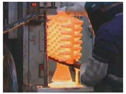
expands and induces great stresses. The mold is then subjected to a *burnout*, which heats the mold between 870 °C and 1095 °C to remove any moisture and residual wax, and to sinter the mold.
