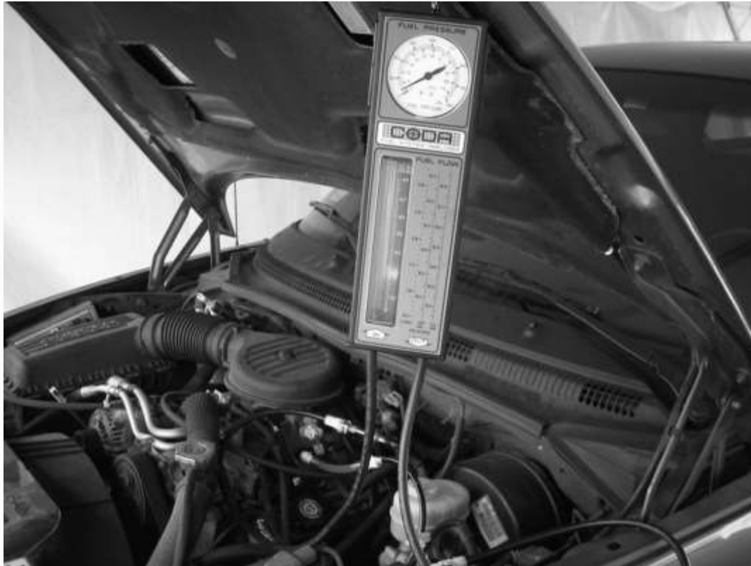
FIGURE 33-27 A fuel system tester connected in series in the fuel system so all of the fuel used flows through the meter which displays the rate-of-flow and the fuel pressure.
