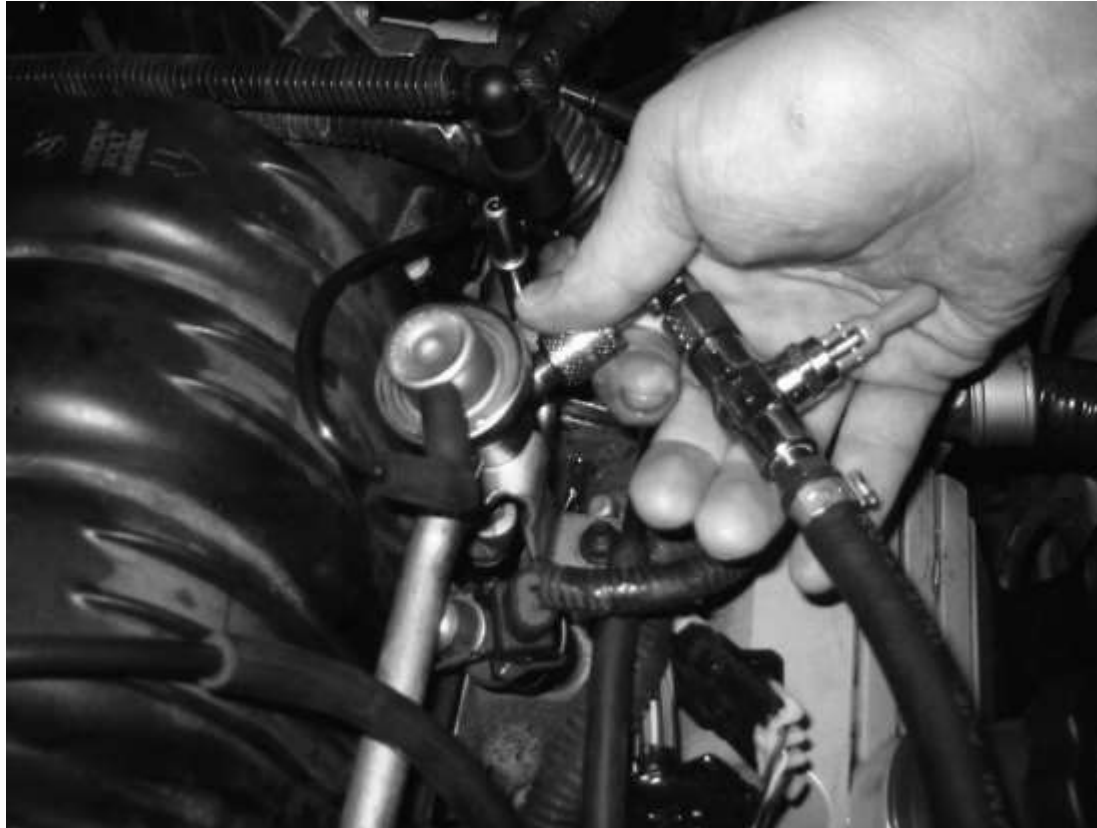
FIGURE 33-22 The Schrader valve on this General Motors 3800 V-6 is located next to the fuel-pressure regulator.
