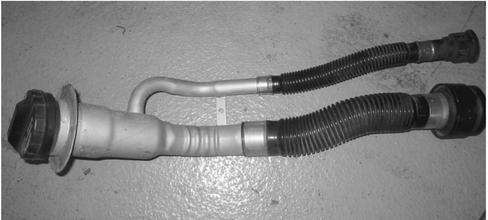
FIGURE 33-4 Vehicles equipped with onboard refueling vapor recovery usually have a reduced size fill tube.
