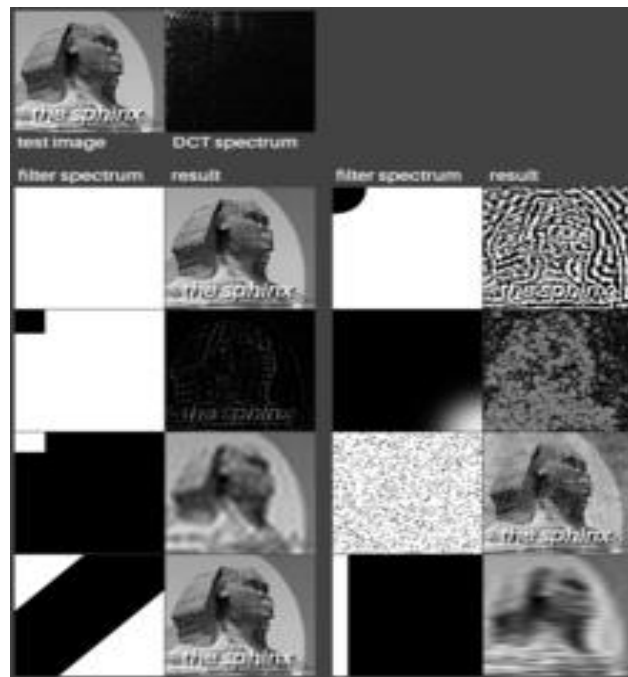
Figure: showing eight different filters applied to a test image (top left) by multiplying its DCT spectrum (top right) with each filter.
