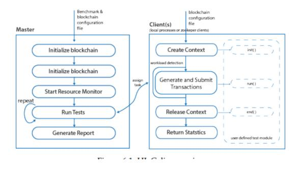
The caliper architecture composed by a master node that orchestrate a pool of client that communicate invoke and query the blockchain implemented for the particular use case.
