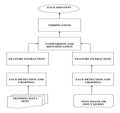
Fig. Architecture Diagram for Proposed Method
