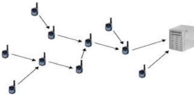
Figure 1. Huge quantities of sensors that carrying information wirelessly to a base station.
