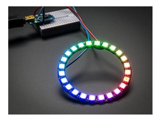
Incorporating scads of LEDs into an electronic project used to be a hairy prospect, a veritable rat's nest of wires and code. The arrival of dedicated LED driver chips brought welcome relief, offloading grunt work from the microcontroller and allowing one to focus on the application. Much simpler, but still not "Christmas light" simple.
