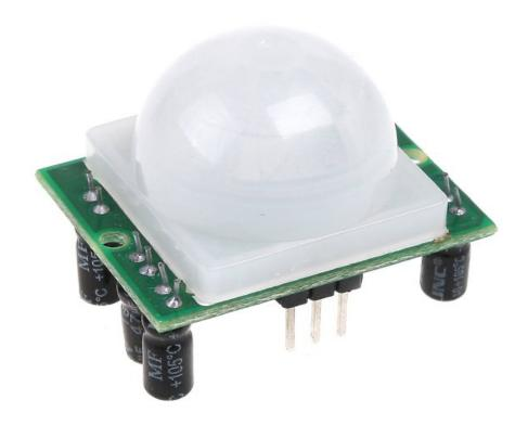
Passive InfraRed sensors can detect movement of objects that radiate IR light (like human bodies). Therefore, using these sensors to detect human movement or occupancy in security systems is very common. Initial setup and calibration of these sensors takes about 10 to 60 seconds.
